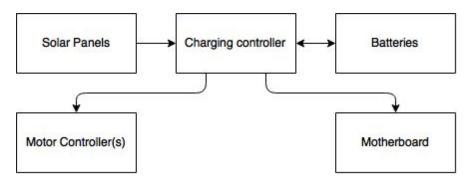
Figure 1: Block diagram of power distribution
