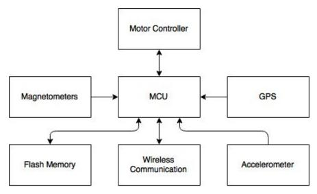
Figure 2: Block diagram of hardware communication signals
