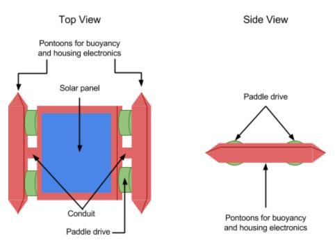
Figure 4: Diagram of potential chassis of drone (not to scale)
